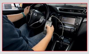
By using the radio remote control it is possible to manage the entire testing procedure. Through the same device, it is possible to transmit the forces applied to the lever (for motorcycles and three-/fourwheelers) or pedal controls to the operating program for the correct measurement of the braking efficiency.
